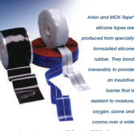
temperature range (-65°F up to +500°F). Our products provide superior electrical insulation with a dielectric strength of 300 VPM minimum at 356°F/180°C.
