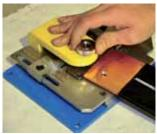
USB STRIPPING TOOL FOR INSULATED FLEXIBLE BAR
