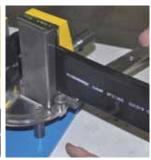
UPB TWISTING TOOL FOR INSULATED FLEXIBLE BAR
